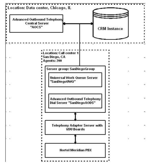
The above diagram shows two interaction centers: one data center and one call center. The data center, which is located in Chicago, houses the CRM database instance and the Oracle Advanced Outbound Telephony Central Server. The call center, which is located in San Diego and has 200 agents, houses 1 instance of the Oracle Advanced Outbound Telephony Dial Server (SanDiegoAdvanced Outbound TelephonyDS). In this example, the call center in San Diego uses a Nortel Meridian PBX.
